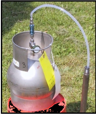
Summa Canister to collect indoor and sub-slab air
