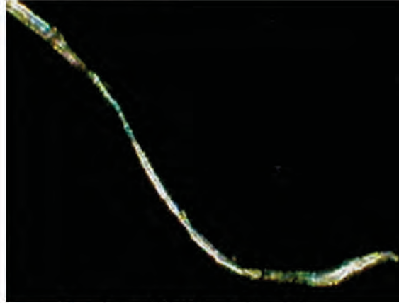
Fiber from USG 5/8 - 15 \mu m width
