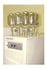
The universal sampling system can provide quantitative and qualitative data for polar, non-polar and reactive volatile organics as well as fixed gases. Detection range extends from 0.5 ppbv to the percent range.
